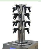
24-Port column manifold for external drying of larger volumes of liquids or slurries in flasks. Includes 24 ports, mounted radially around column with 24 removable neoprene valves, each of which can be fitted with a flask of up to 1 litre capacity (flasks not supplied). A manifold sealing gasket is provided with to seal the base.
