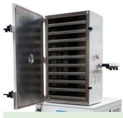
SS freeze drying chamber, with 10 removable trays each measuring 450mm wide x 345mm deep. With single viewport. Available unheated as standard, or with optional heating (part number LSCC10H). With optional manifold ports if required. Compatible with LyoDry Midi or LyoDry Midi Pro
