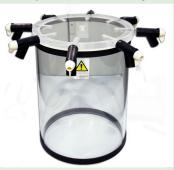
Multipurpose freeze drying chamber for bulk and flask drying comprising: Acrylic drying chamber: 350mm dia x 435mm high, and 2 x L-gaskets, with 8-port valve lid, including 8 x removable, neoprene vacuum isolation valves, 3/4" ID Part No: LSAD6H Acrylic Drying Chamber with 6-Tray Rack Assembly, Heated
