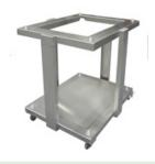
Purpose built SS trolley with castors and brakes, and bottom shelf to accommodate vacuum pump. Specially designed to be lower than a standard lab bench for easy access to drying chamber. With 2 x fixed castors and 2 x swivel castors with brakes
