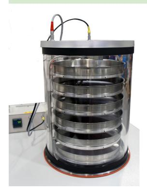
The LyoDry Heated Tray Drying Accessory - part number LSAD6H - is one of <u>a range of freeze drying accessories</u> designed for use with LyoDry Benchtop and Midi freeze dryer condensers.
